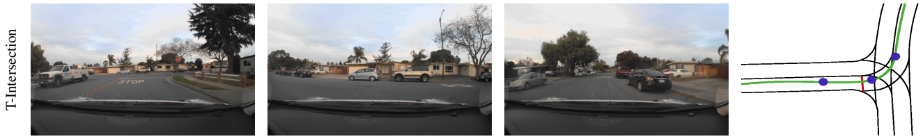
Fig. 3. Experiments demonstrating MODIA on a fully operational autonomous vehicle prototype at a T-intersection. The right three figures show the abstract map (black), stop line (red), path (green), and points along the route (blue) corresponding to each of the three pictures to its left.
