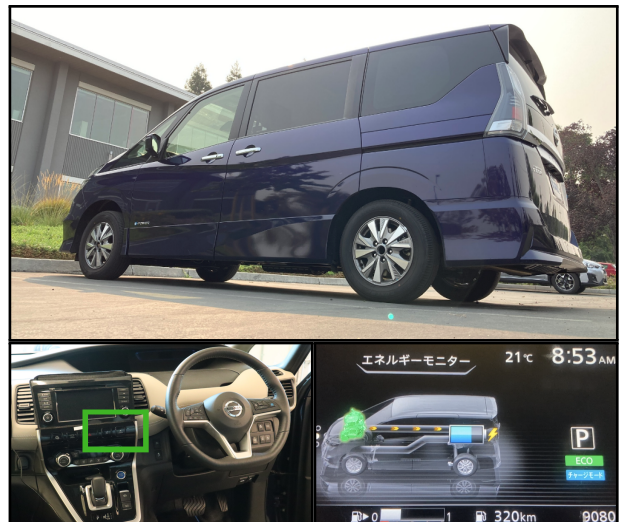
Fig. 3. The 2018 Nissan Serena vehicle used in the experiments (top). The manual control buttons are also highlighted in green (bottom left). They are triggered electronically in the experiments, such as activating charge mode (bottom right). Figure 1 shows experimental results on this real vehicle.
