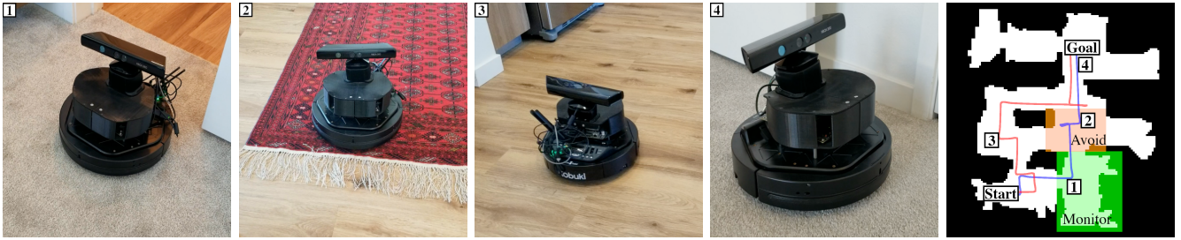
Fig. 3. Experiments that implement home navigation on a real robot in an actual household environment. This uses the M \rightarrow A \rightarrow G DAG with two paths: (1) constrained-to-monitor (blue path) with \eta_1 = \eta_2 = 0 , and (2) constrained-to-avoid (red path) with \eta_1 = 100 and \eta_2 = 0 . The start point (S), goal point (G), avoid region, and monitor region are shown.
