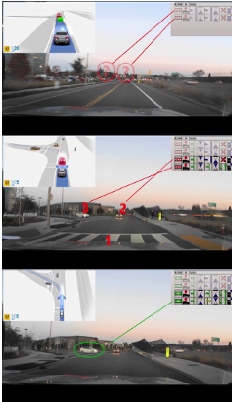
Figure 7.4: Experiment 3-Way Stop (Part 1 of 2) in Sunnyvale, California during 2017. This is MODIA, as part of a policy network, interacting with real traffic on a public road. The left corner shows a visual of the high-level route plan. The right corner shows a visual of the mid-level MODIA decision-making; each row represents one DC. Images provided courtesy of Nissan Research Center - Silicon Valley.
